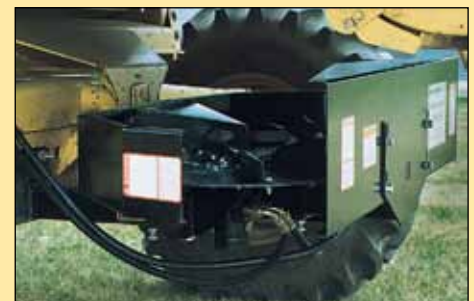
Cyclones come complete with hydraulic motor, hoses, fittings, flow valve and flow pans (where needed).
